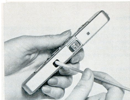
Clean lens window with cotton swab-or with a clean linen cloth wrapped around a match or wood stick.
